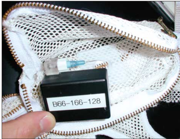
Figure 3. Oxygen generation device (Ogenix Corp, Cleveland, Ohio) secured in body-mounted harness.
